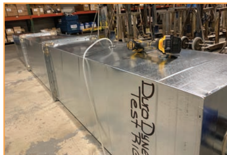
Heritage Mechanical built a test rig to test leakage for the EZ corners. They tested to 6" wg and had zero leakage and pushed to 8" wg with 0 leakage.
