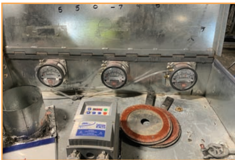
Heritage Mechanical built a test rig to test leakage for the EZ corners. They tested to 6" wg and had zero leakage and pushed to 8" wg with 0 leakage.
